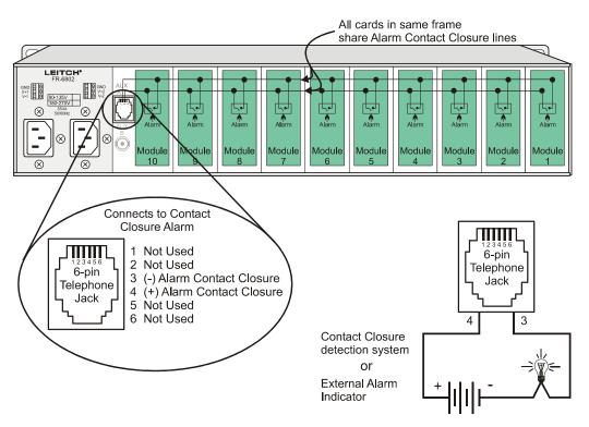
Figure 1-5. External Alarm Connections
